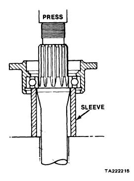
Figure 11-48. Shaft and Bearing Removal
