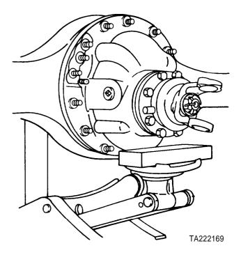
Figure 11-2. Carrier Removal
