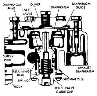
Figure 9C.5. Relay Valve (36Z291)
