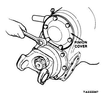
Figure 11-180. Securing Pinion Cover
