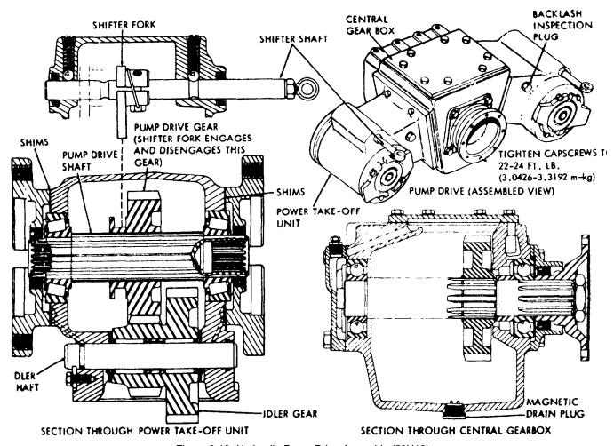
Figure 8-13. Hydraulic Pump Drive Assembly (53U13)
