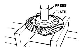
Figure 11-91. Press Case from Gear
