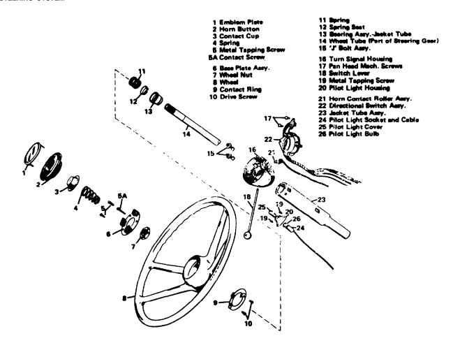
Figure 10-5. Steering Column (20Z1144)
