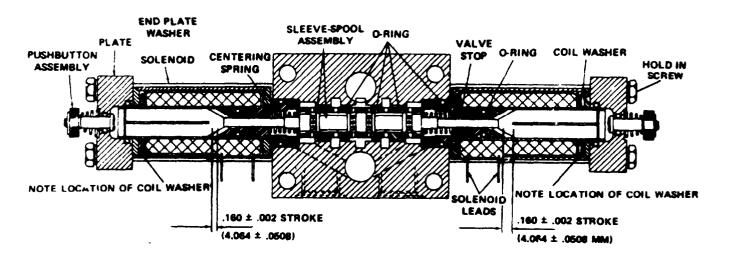
Figure 7-4. Solenoid Operated Valve (36Z341)
