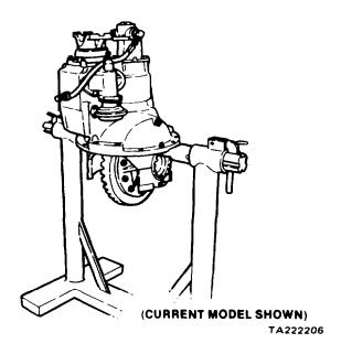
Figure 11-39. Carrier Mounted in Holding Fixture
