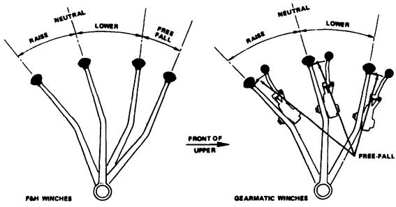
Figure 2-8. Winch Lever Positions
