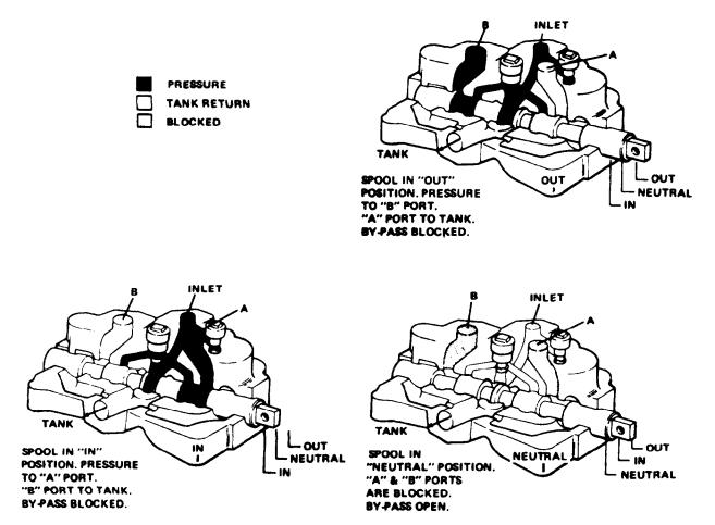
Figure 4D-9. Control Valve Operation (36Z986)
