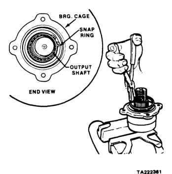
Figure 11-194. Installing Bearing Retainer
