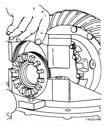
Figure 11-23. Installing Differential Assembly
