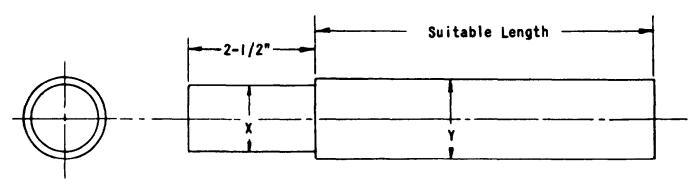
Dimension X" is 0.010" less than the bushing bore. Dimension Y" is 0.010" less than the steerling knuckle bore.
