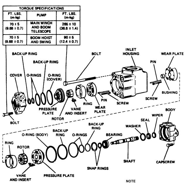
A CARTRIDGE KIT CONSISTS OF A PRESSURE PLATE, ROTOR, VANE KIT AND INSERTS, RING WEAR PLATE, TWO PINS, AND TWO SCREWS.
