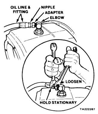
Figure 11-100. Disconnecting the Oil Lines
