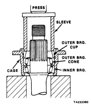
Figure 11-193. Installing Outer Bearing Cup
