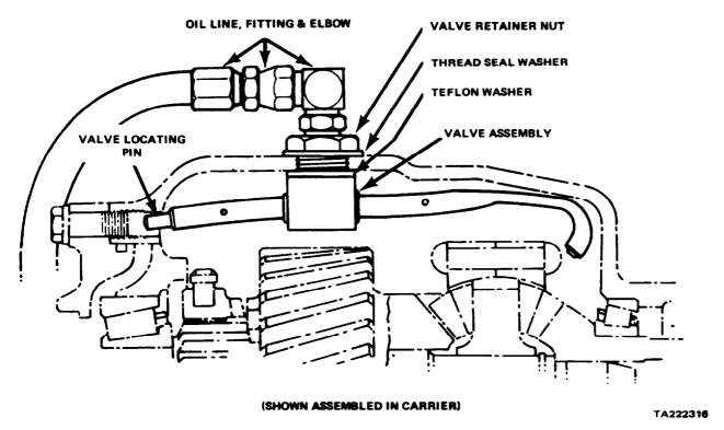
Figure 11-149. Oil Valve in Carrier
