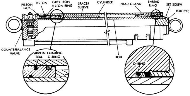
Figure 5C-1. Boom Telescope Cylinder
