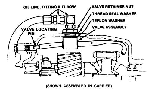
Figure 11-99. Oil Valve Assembly
