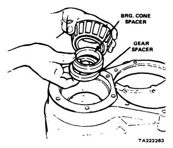
Figure 11-96. Removing Pinion Shaft Components
