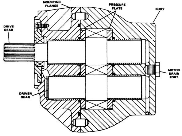
Figure 5K-1. Winch Motor (41Q6)
