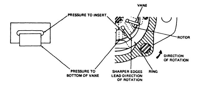
Figure 4B-16. Pressure Feed to Vanes
