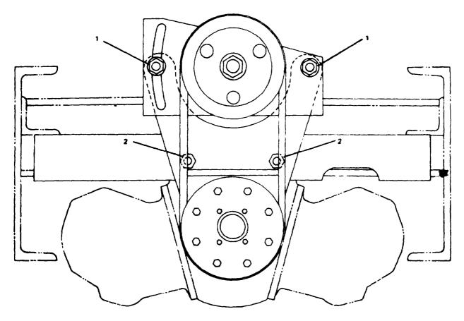
Figure 8-14. Power Steering Pump Installation
