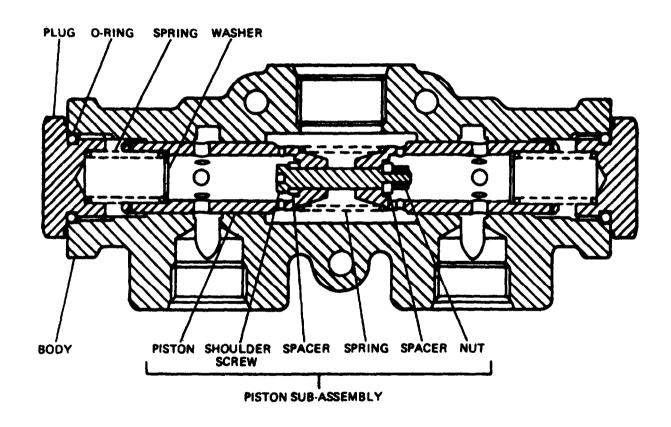
Figure 5D-4. Flow Divider (36Q46)
