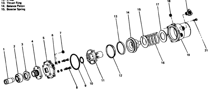
Figure 9C-16. Throttle Valve (36U29)
