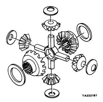
Figure 11-20. Differential Gears and Washers
