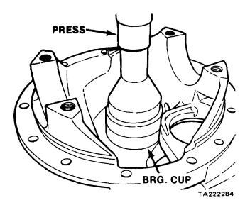
Figure 11-117. Installing Bearing Cup
