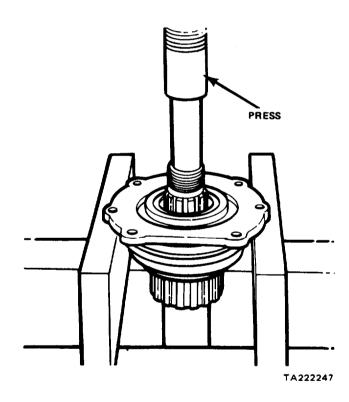
Figure 11-80. Input Shaft Removal
