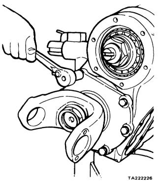
Figure 11-59. Input Shaft Bearing Cage Removal
