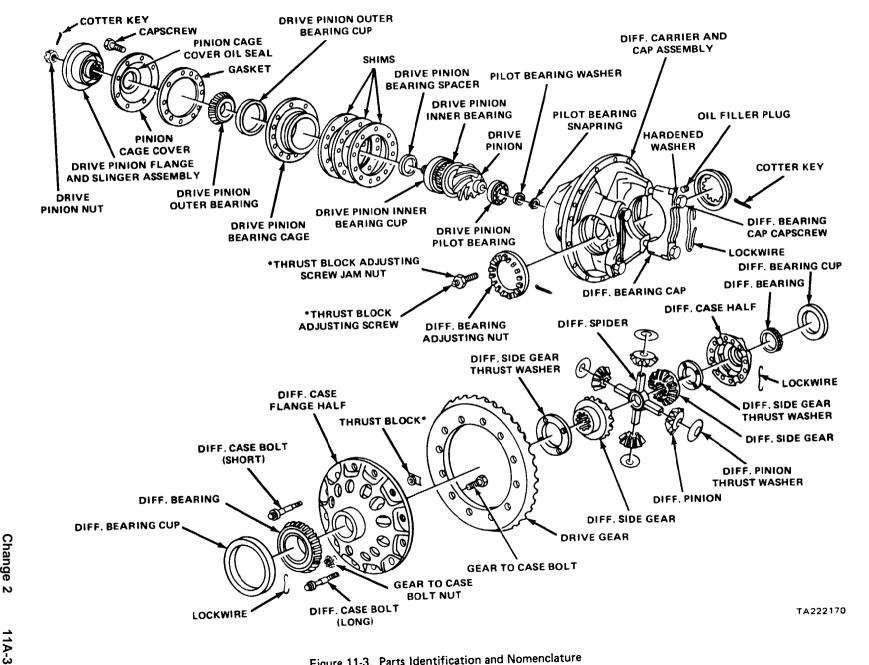
Figure 11-3. Parts Identification and Nomenclature
