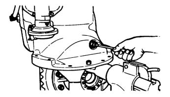
Figure 11-40. Thrust Block Jamnut
