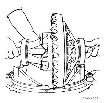
Figure 11-7. Removing Differential and Gear Assembly
