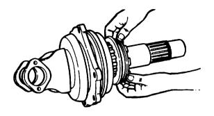
Figure 11-78. Clutch Collar Removal
