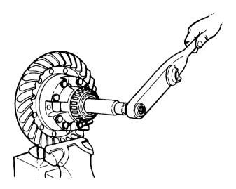
Figure 11-126. Torquing Differential Nest
