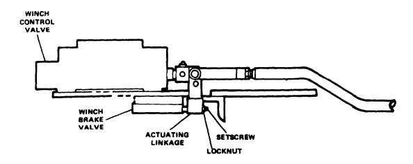
Figure 5H-4. Linkage Adjustment
