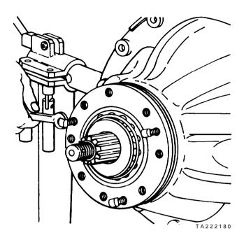
Figure 11-13. Bearing Cage Removal
