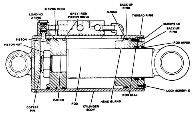
Figure 5B-1. Boom Hoist Cylinder (38Z231)
