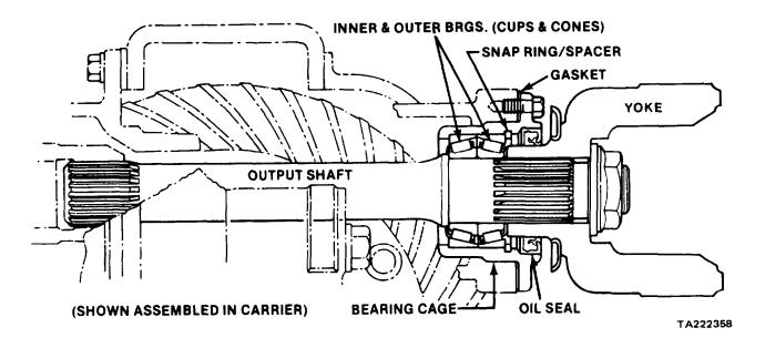
Figure 11-191. Current Model Tapered Bearings
