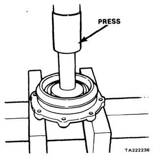
Figure 11-69. Oil Seal Removal
