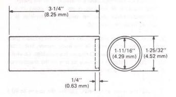
The driver can be made from tubular stock machined to the
