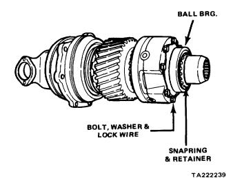
Figure 11-72. Rear Side Gear Assembly
