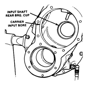
Figure 11-167. Installing Rear Bearing Cup
