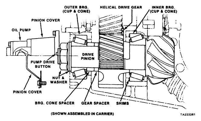
Figure 11-94. Drive Pinion Assembly
