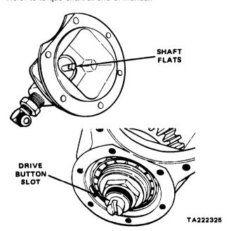
Figure 11-158. Pump Shaft Alignment
