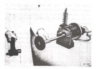
Figure 9D-8. Removing Push Rod Bushing
