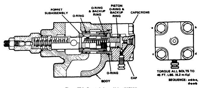
Figure 5F-3. Counterbalance Valve (36Z683)
