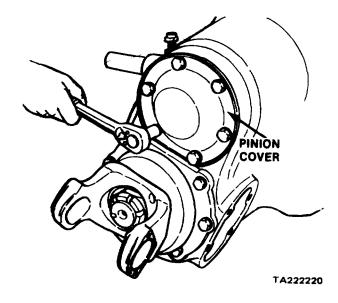
Figure 11-53. Pinion Cover Removal, Original Model
