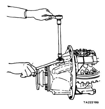
Figure 11-32. Adjusting Screw Installation
