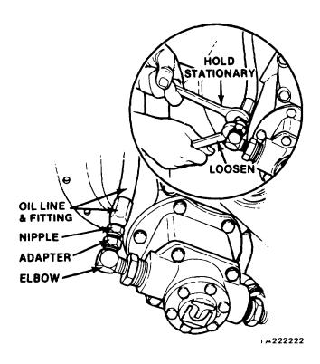
Figure 11-55. Disconnecting Oil Lines
