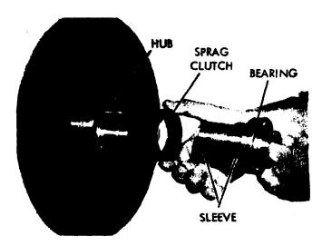
Figure 7. Removing Sleeve and Sprag Clutch
