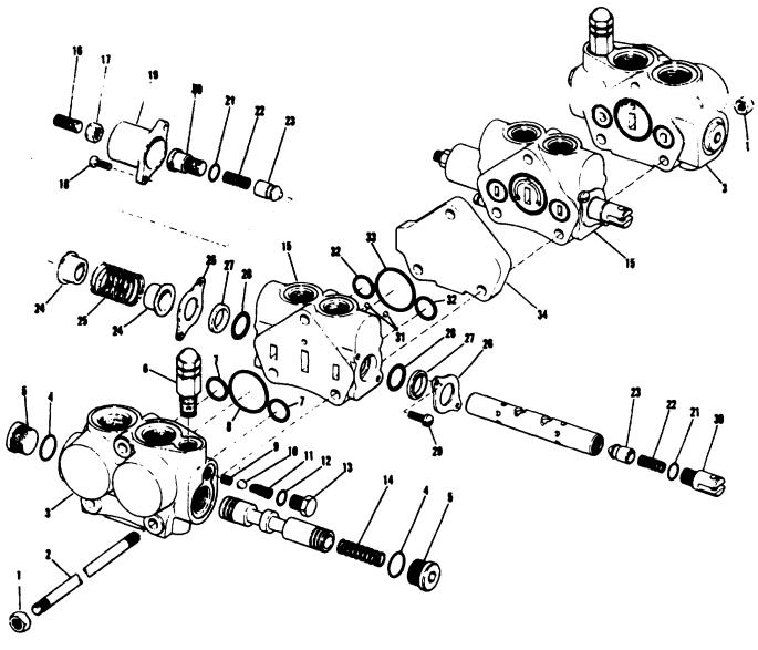
Figure 4D-15. Control Valve (36Z840)
