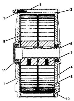
Figure 5E-2. Hose Reel Spring Motor
