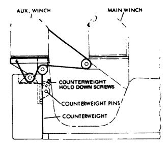
Figure 2-19. Counterweight Removal (1002382)
