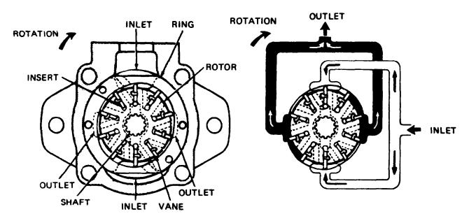
Figure 4B-37. Pump Cartridge Operation
