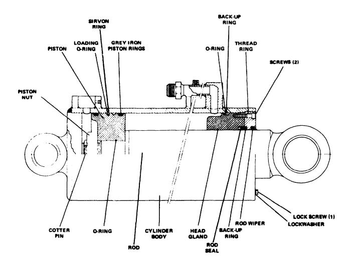
Figure 5B-2 Boom Hoist Cylinder (38U92)
