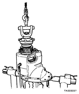
Figure 11-60. Inter-Axle Differential Removal
