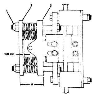
Figure 5J-22. Dimensions for Spring Setting
