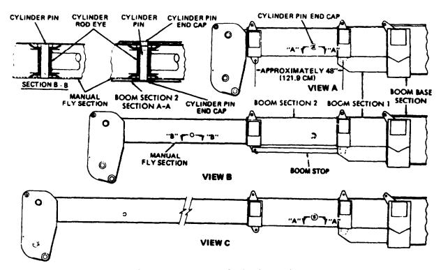
Figure 2-18. Manual Fly Section (105J681)
