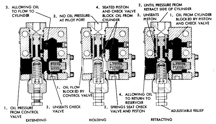
Figure 5F-7. Counterbalance Valve Operation
