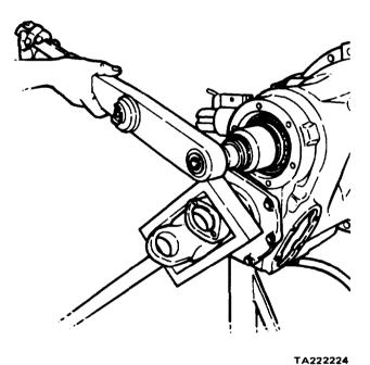
Figure 11-57. Pinion Nut Removal
