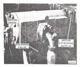
Figure 5K-8. Motor Removal
