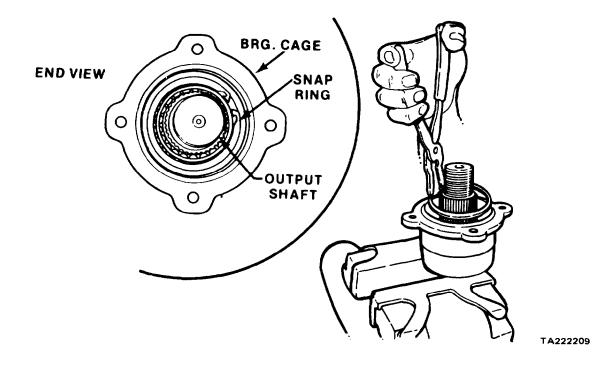
Figure 11-42. Removing Snapring
