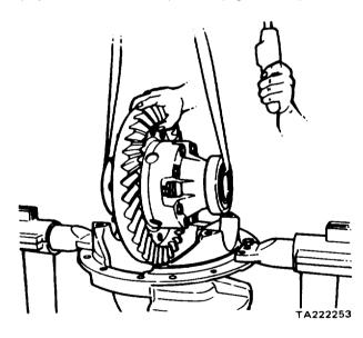
Figure 11-86. Removing Differential and Gear Assembly D. Using a suitable and safe lifting fixture, lift out the main differential and gear assembly from carrier (Figure 11-86).
