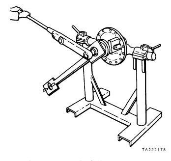
Figure 11-11. Removing Shaft Nut and Washer
