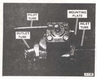
Figure 5F-5. Counterbalance Valve Removal
