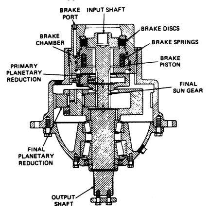
Figure 6D-1. Swing Transmission (53R3)
