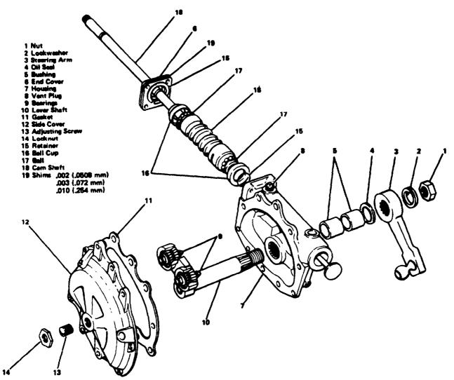
Figure 10-6. Steering Gear (53Z341)
