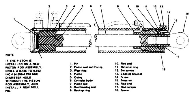
Figure 7-5. Outrigger Extension Cylinder (10053305)
