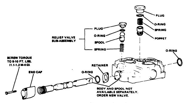
Figure 4D-10. Control Valve (36Z986)
