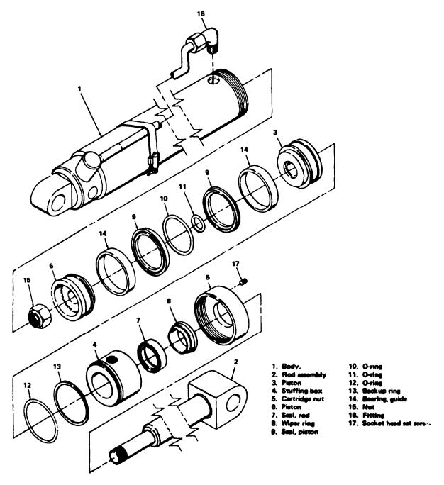
Figure 7-6. Outrigger Extension Cylinder (38489 & 38491)
