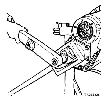
Figure 11-58. Input Shaft Flange Nut Removal
