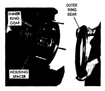
Figure 14. Removing Outer Ring Gear
