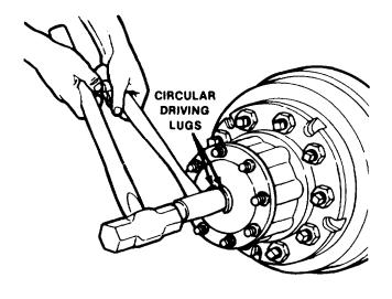
Figure 11-38. Removing Axle
