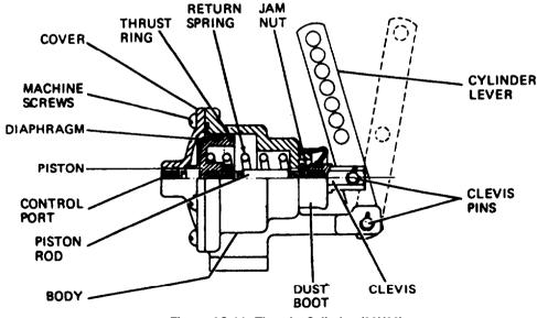
Figure 9C-14. Throttle Cylinder (36U30)
