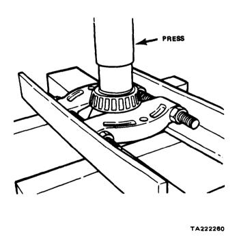
Figure 11-93. Removing Cone
