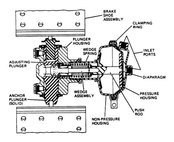
Figure 90-1. Front Brake Mechanism
