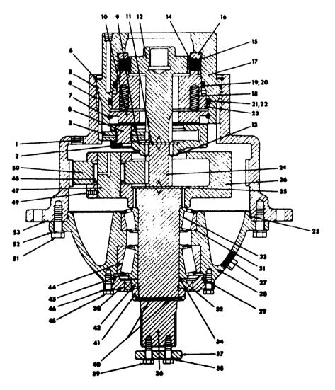
Figure 6D-3. Swing Transmission (53R3)
