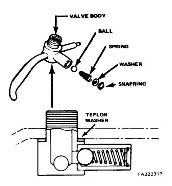
Figure 11-150. Valve Body Parts
