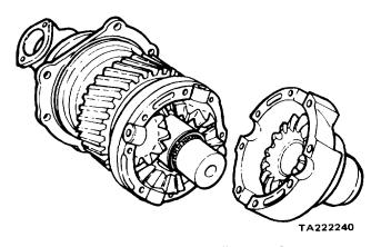
Figure 11-73. Inter-Axle Differential Case
