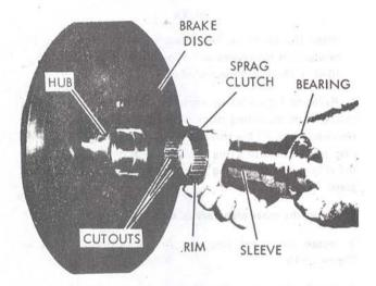
Figure 5J-18. Installing Sprag Clutch
