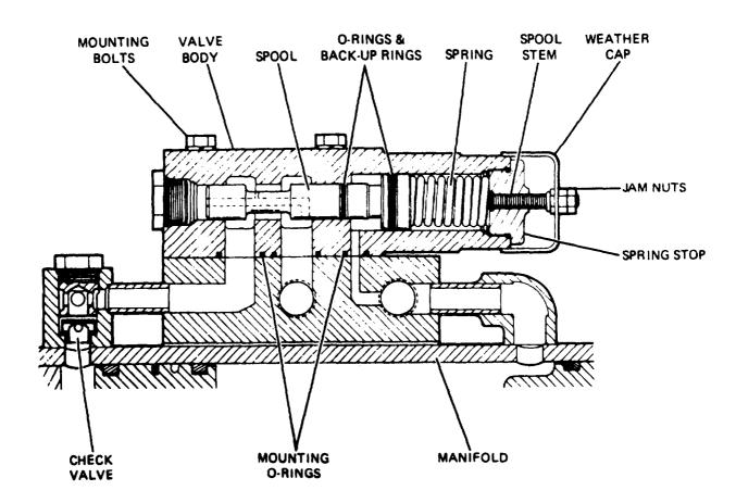
Figure 5G-2. Velocity Fuse (1036Z403)
