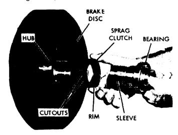
Figure 17. Installing Sprag Clutch
