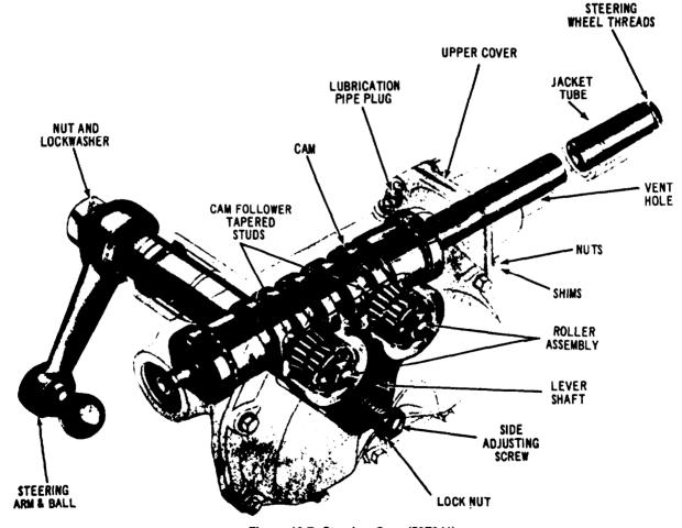
Figure 10-7. Steering Gear (53Z341)
