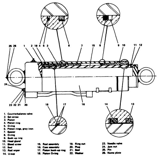
Figure 5C-3. Boom Telescope Cylinder (38R32)
