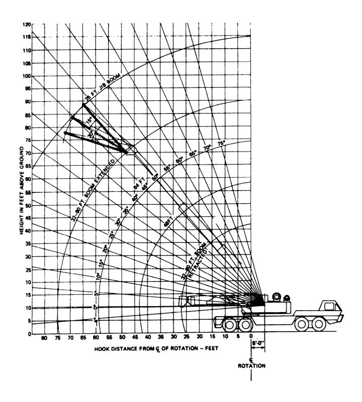
Figure 1-3. Range Diagram - 80' Boom (105x75-A)
