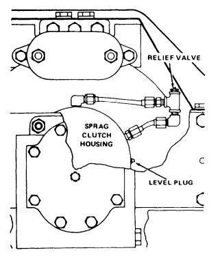
Figure 5J-20. Sprag Clutch Oil Level
