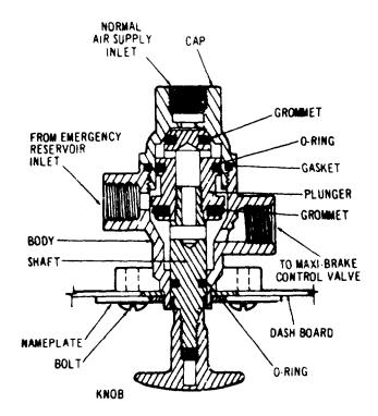
Figure 9C-9. Emergency Release Valve (362362)
