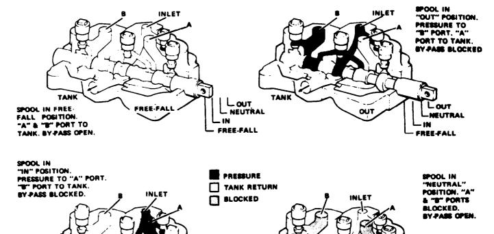
Figure 4D-11. Control Valve Operation (36Q70)
