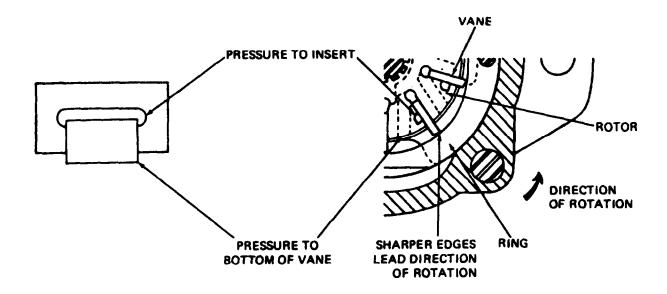
Figure 4B-3. Pressure Feed to Vanes
