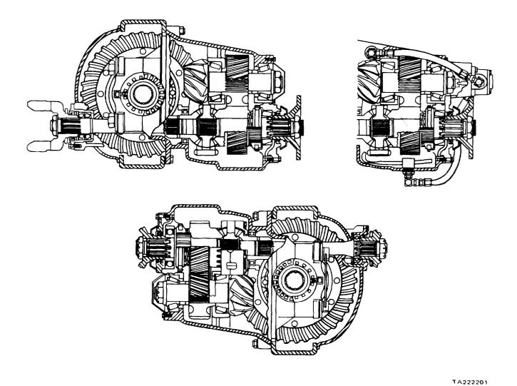
Figure 11-34. Front Mounted Single-Reduction Drive Units
