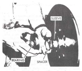
Figure 5J-19. Bearing and Spacer Location
