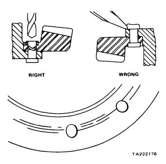
Figure 11-9. Removing Gear Rivets
