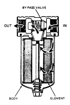
Figure 4E-1. Filter Operation
