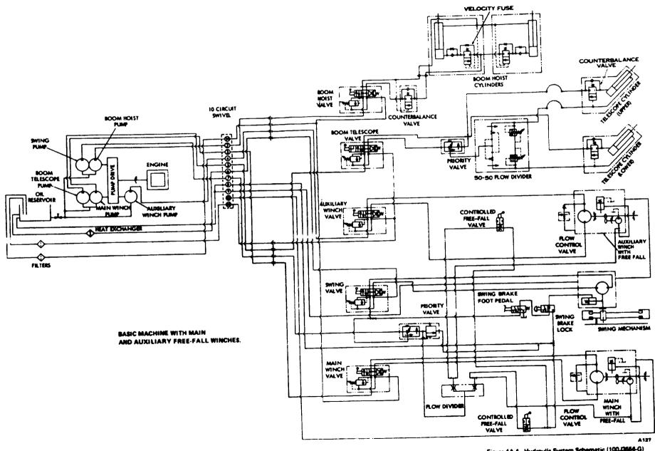
Figure 4A-4. Hydraulic System Schematic (100.03666-G)
