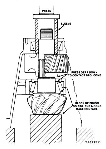
Figure 11-144. Installing Helical Gear
