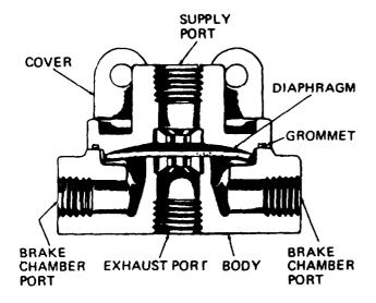
Figure 9C-4. Quick Release Valve (36Z254)
