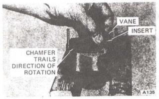
Figure 4B-12. Installing Vanes and Inserts
