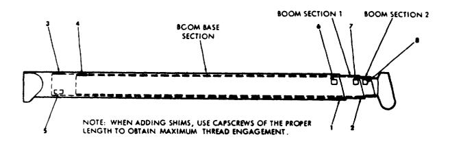
Figure 5A-3. Boom Alignment (1100P154)
