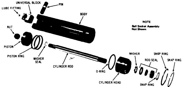
Figure 10-15. Steering Cylinder (45Z265)
