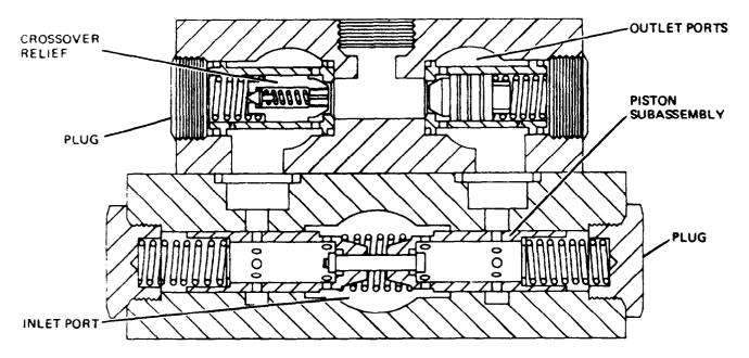
Figure 5D-2. Flow Divider (36Z680)
