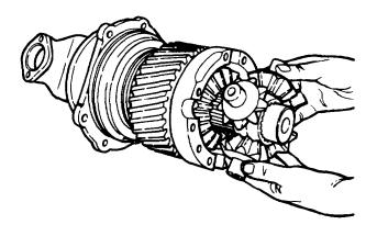
Figure 11-172. Installing Spider Assembly
