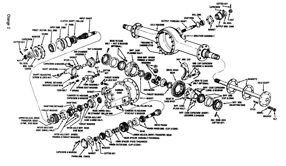
Figure 11-37. Typical Original Drive Unit
