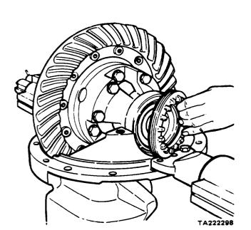
Figure 11-131. Installing Bearing Adjusting Rings
