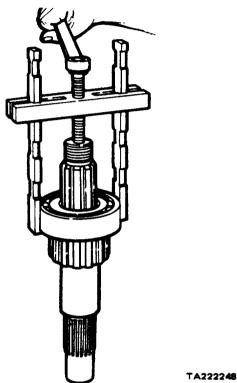
Figure 11-81. Ball Bearing Removal
