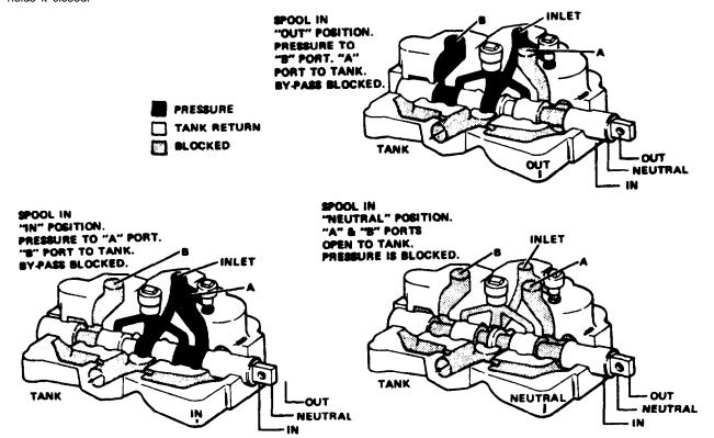
Figure 4D-1. Control Valve Operation (36Z724)
