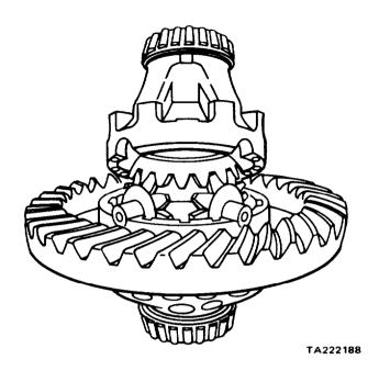
Figure 11-21. Differential Case Assembly
