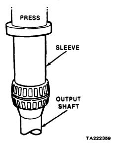
Figure 11-192. Installing Inner and Outer Cones **NOTE**
