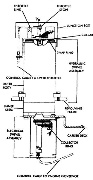
Figure 4C-1. Rotary Joint (979J24)
