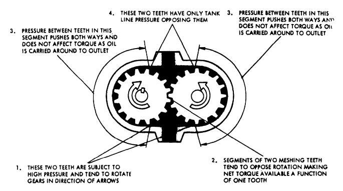
Figure 6C-1. Swing Motor Operation
