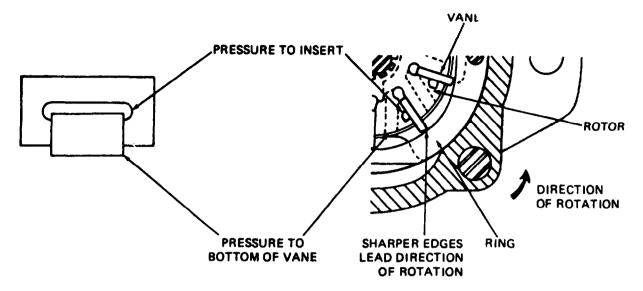
Figure 4B-38. Pressure Feed to Vanes
