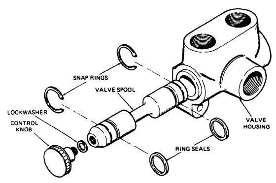
Figure 10-3. Steering/Outrigger, Selector Valve (36Z706)
